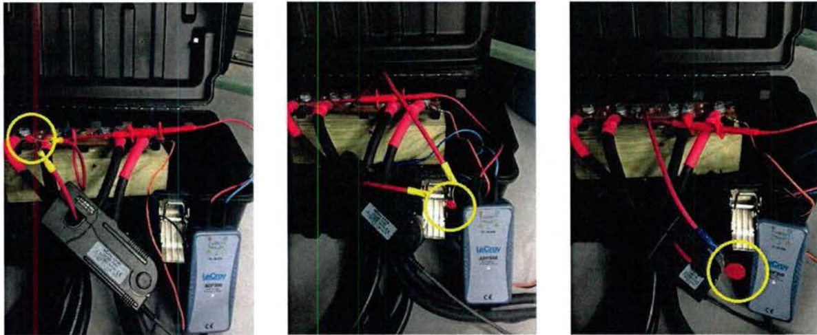
Figure 21: The V10E23P placed parallel to the bus with the differential voltage probes and the clamped-on current meter (left) the V07E30P with the same exact set up (middle) the V20E35P also with the same exact set up (right).
