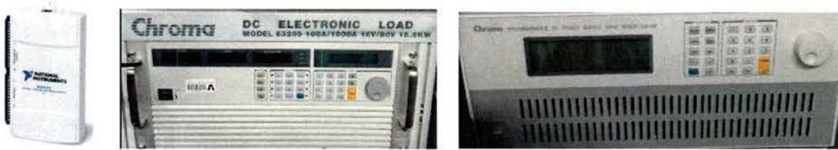
Figure 7: The NI-USB-6211 multifunction IO device used to control the load and supplies (left) the Chroma load used for discharge current (middle) one of the two Chroma supplies used for the charge current (right).
