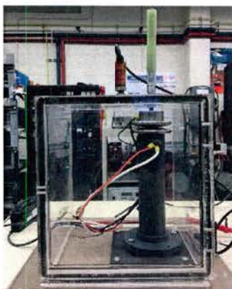
Figure 43: Sealed acrylic chamber containing electrodes used to induce voltage breakdown.
