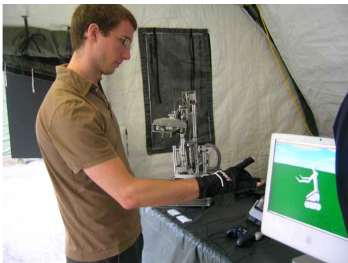
Figure 14. iGlove controlling BEAR arm joints.
