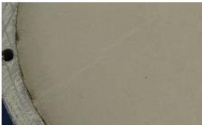
(a) Cracked potting
