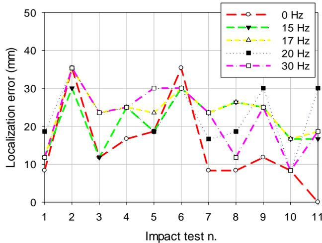
Fig. 4: Impact localization of composite wing under simulated noise conditions.
