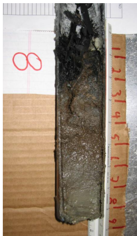
Figure 5-7 Soil Core Collected from APG-08 at Time 0. Photographic scale is in inches.
