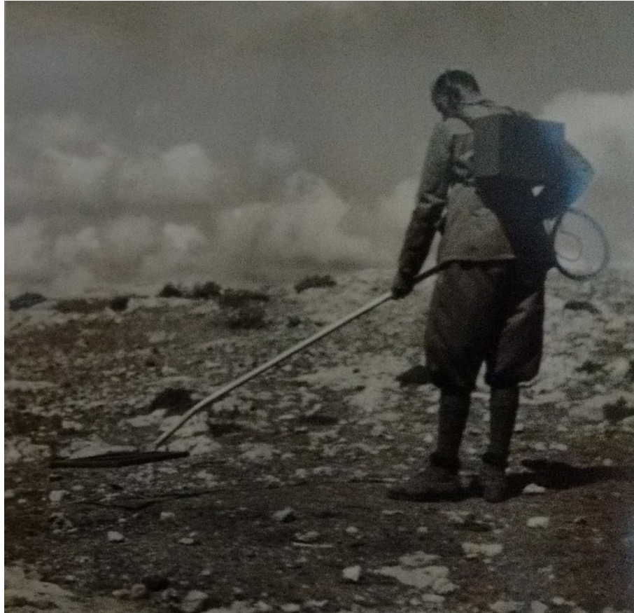
Figure 12. An Italian Soldier using the Mine Detector Model “M”
