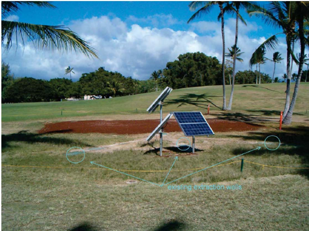
Figure 2. Pilot-Scale Bioreactor Solar Panel at Site LF05 JBPHH, HI
