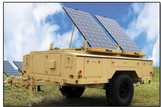
Figure 1: T-Series mobile hybrid power system
