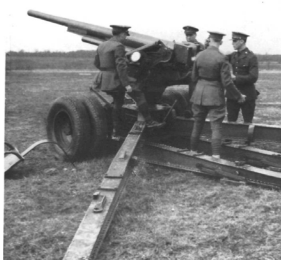
Figure 8: T3 gun mount in 90 degree firing mode. The split trail setup allowed for greater traverse and tube elevation than a box trail setup allowed. G.M. Barnes, "Division Artillery in the Next War" The Field Artillery Journal , Frontispiece.
