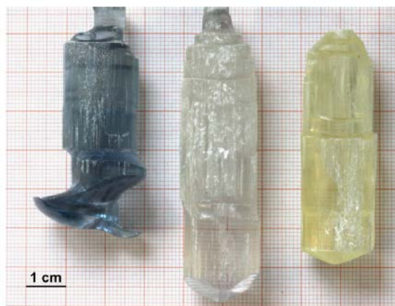
Figure 24: \beta -Ga 2 O 3 Single Crystals Obtained by the CZ Method Carrier concentration 2 \times 10^{18} \text{ cm}^{-3} (left), 4 \times 10^{16} \text{ cm}^{-3} (middle) and insulating with Mg doping (right) [65].
