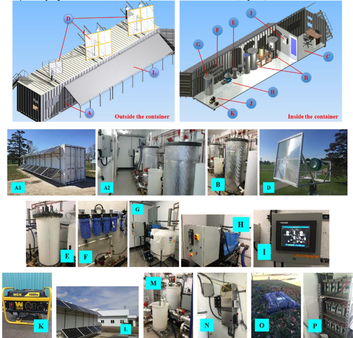
Figure 16. The self-sustaining pilot-scale system
