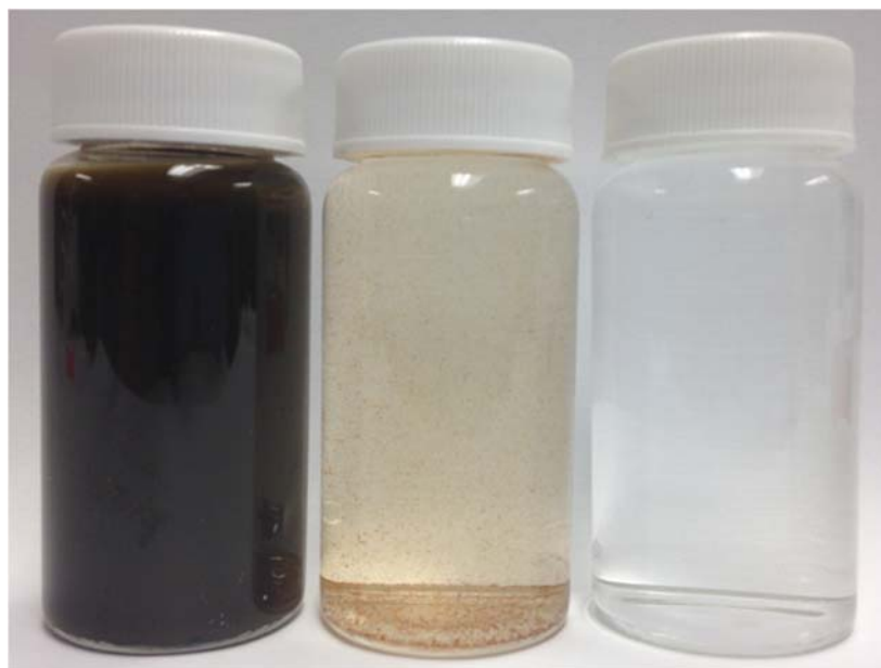
Figure 50. Color change of the solution following different treatment stages Left to right: AD effluent, EC effluent and membrane filtrate.
