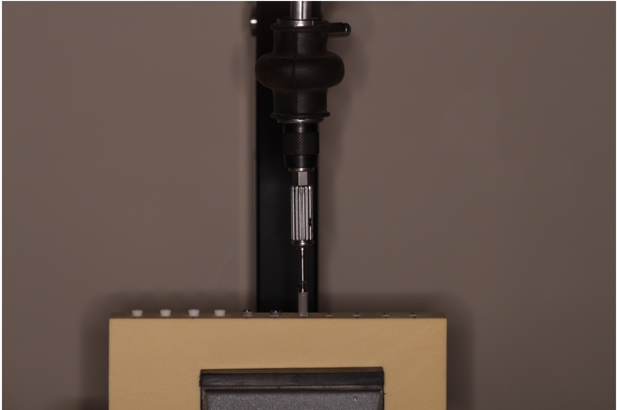
Figure 10: Implant placement with IM-Teknik removal torque machine
