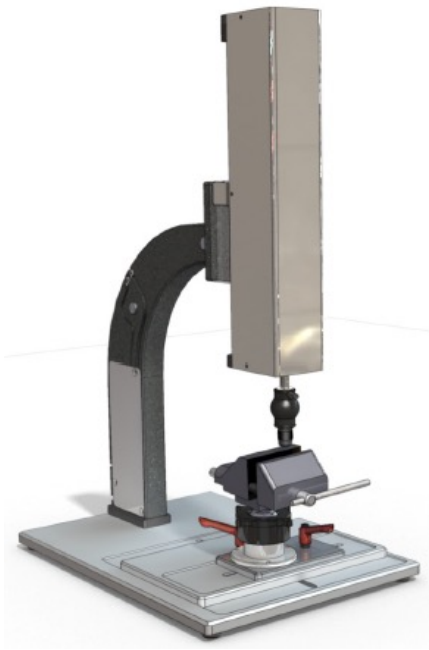
Figure 5: Removal torque measuring device developed and manufactured by IM-Teknik Development AB. Used to place implants with continuous measurement of insertion torque.
