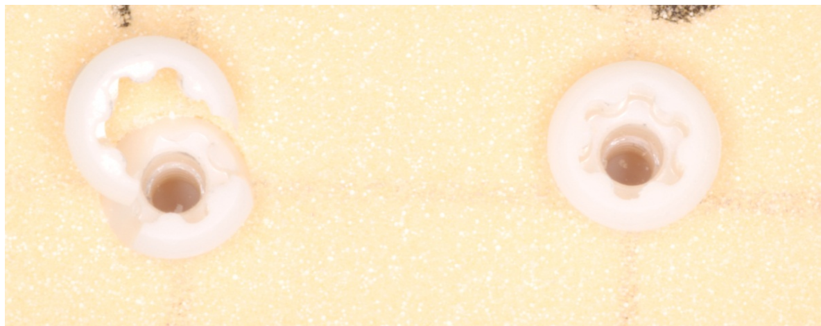
Figure 3: Image depicting fractured Axis Biodental implant
