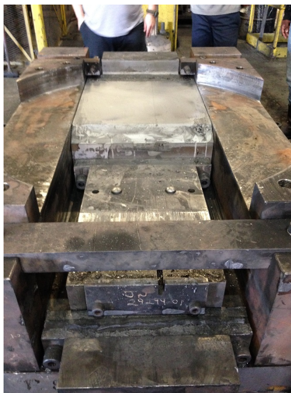
Fig. B-40 Interior arrangement of the components in the base assembly of the ECAE tool with the ring assembly removed
