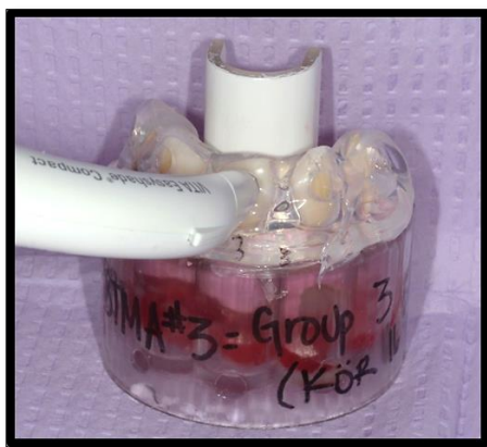
Figure 4. Clear custom stent to standardize placement of spectrophotometer tip
