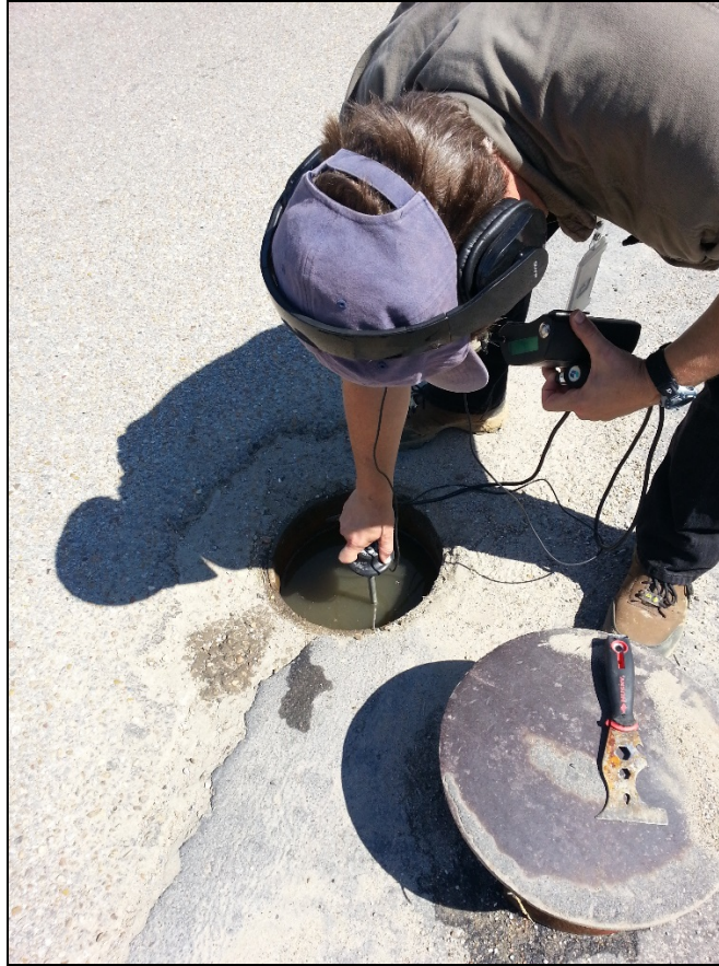
Figure 6-5. Water-filled Valve Box in Vicinity of Leak Detected by ZoneScan Alpha System
