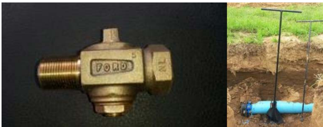
Figure 5-2. Simulated Leak Configuration Using Corporation Valves
