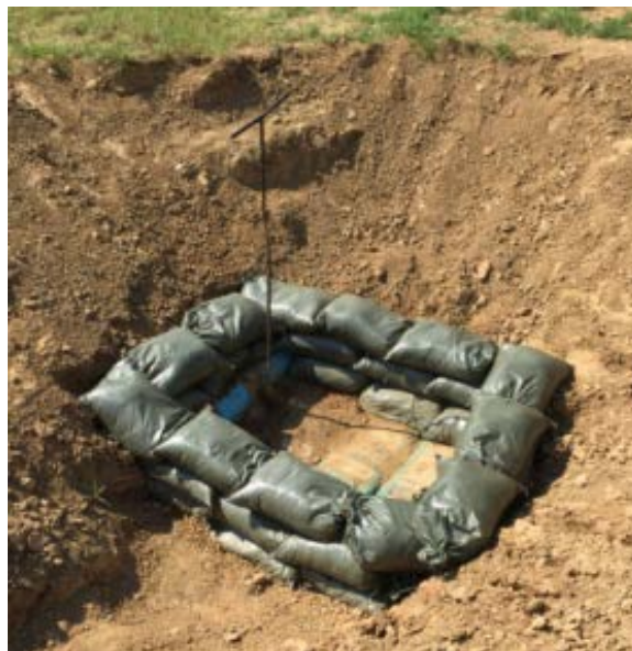
Figure 4-5. Long PVC Run Simulated Leak Pit
