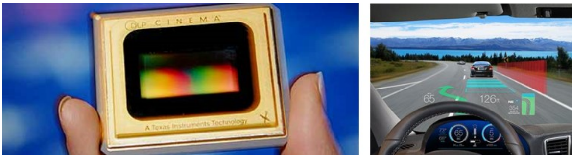
Figure 85: Texas instruments DLP™ and its application in automobile heads-up displays.
