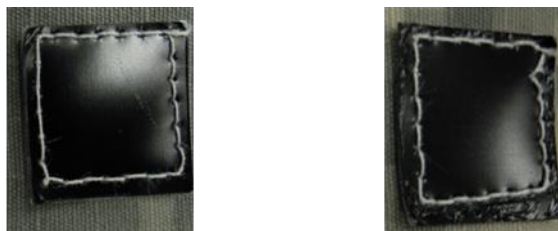
Figure 14. TMET Work Order Number 14412, Part 5, test specimens after five accelerated laundering cycles. a) specimen "A1-Group 2"; b) Specimen "A2-Group 2"
