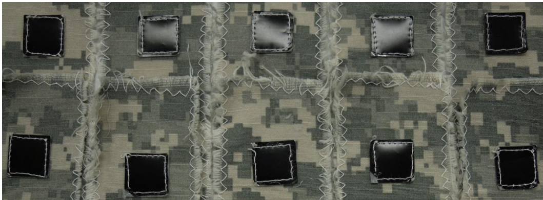
Figure 15. TMET Work Order Number 14412, Part 6, specimens after five accelerated laundering cycles. Top row, left to right: specimens 2, 4, 5, 7, and 8; bottom row, left to right: specimens 11, 12, 13, 14, and
