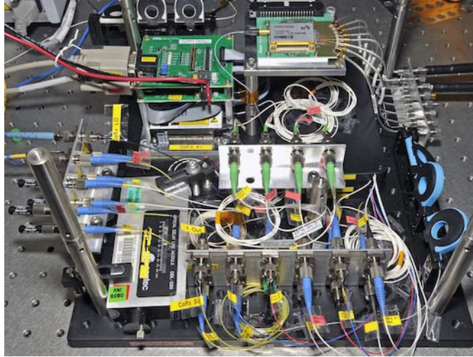
Fig. 6. Photo of a single preamplified coherent receiver mounted on a 12" x 12" optical breadboard.
