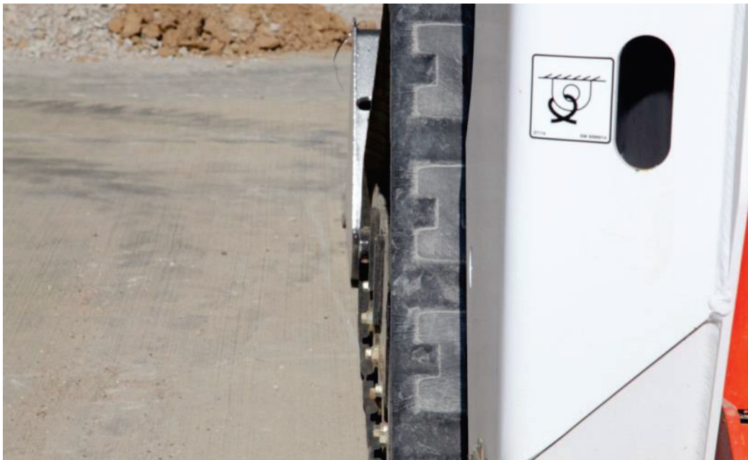
Figure 30. View from rear of Bobcat MT 85 showing width of bucket equal to track width.
