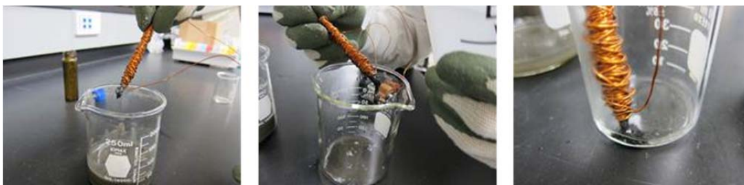
Figure 5. Separation of CCMPs from sediment slurry. Left: collection from the sediment slurry, center: washing the collected particles with deionized water, right: collection of washed particles.
