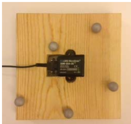
Figure 8. Mounted 3DM-GX4-25 with Infrared Markers for Posture Detection
