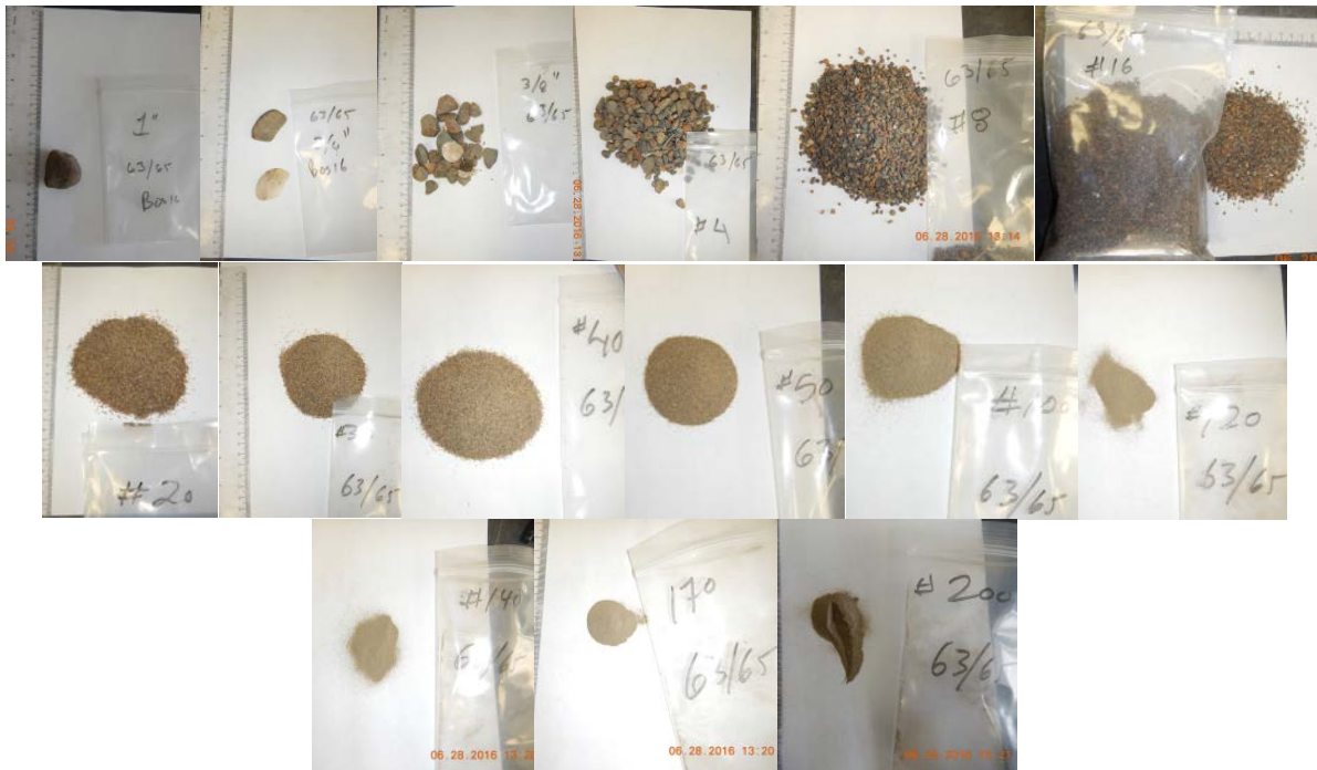
Fig. 6 Sample 3 (positions 63, 65) “SPg” – grain-size by sieve (retaining): 25.4, 19, 9.5, 4.75, 2.36, 1.18, 0.85, 0.6, 0.425, 0.3, 0.15, 0.125, 0.106, 0.09, 0.075 mm.
