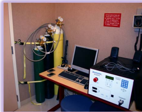
Figure 1. The reduced oxygen breathing device and tanked gases used to generate normobaric hypoxia.
