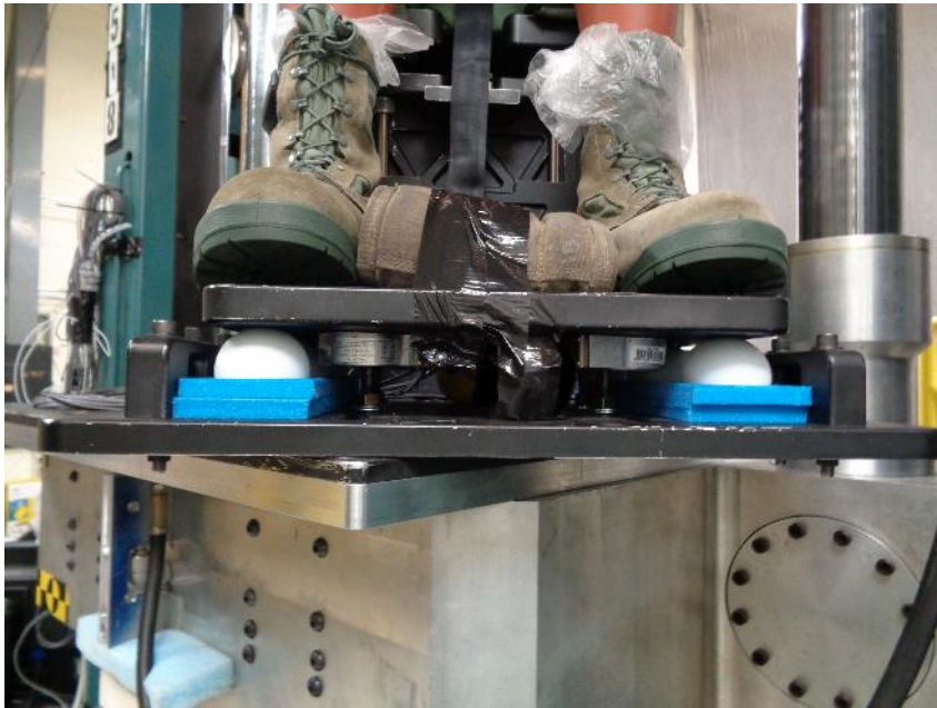
Figure 12. Foot-Rest Programmer (White Elastic Lacrosse Balls) Used for Test Series 3
