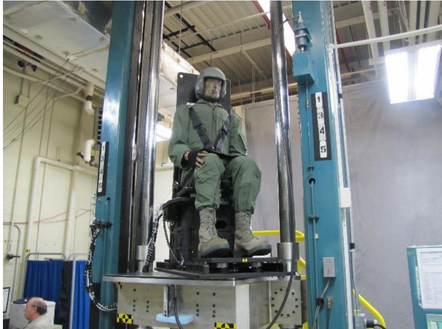
Figure 2. VID with WIAMan Seat Two (WS2) Mounted on Top of Carriage: Front View
