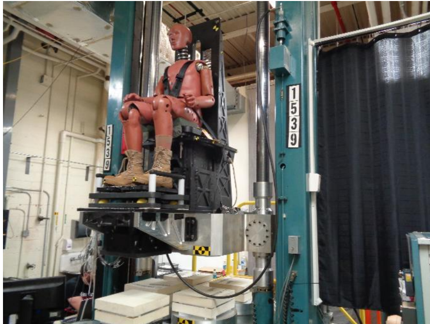
Figure 7. WS3 Seat Fixture Orientation of VID With Hybrid III Manikin
