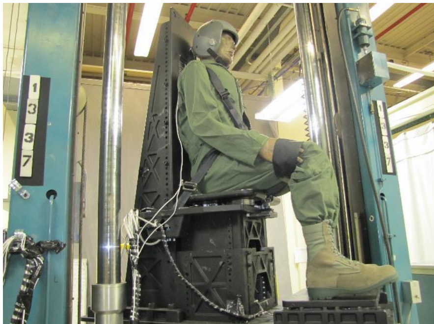
Figure 3. VID with WIAMan Seat Two (WS2) Mounted on Top of Carriage: Side View
