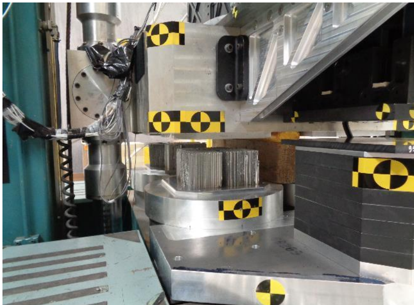
Figure 13. Carriage Programmer (Hexcel) Used for Test Series 4
