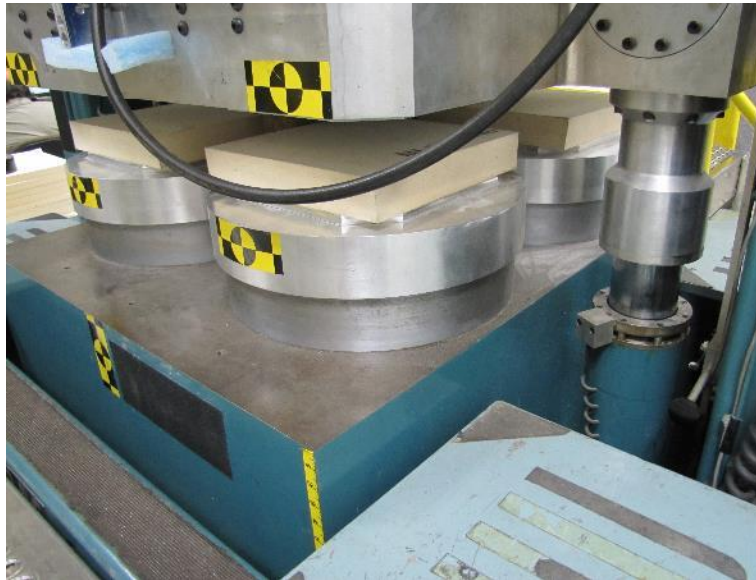
Figure 10. Carriage Felt Programmers (2" Thick Single Layer) used for Test Series 1
