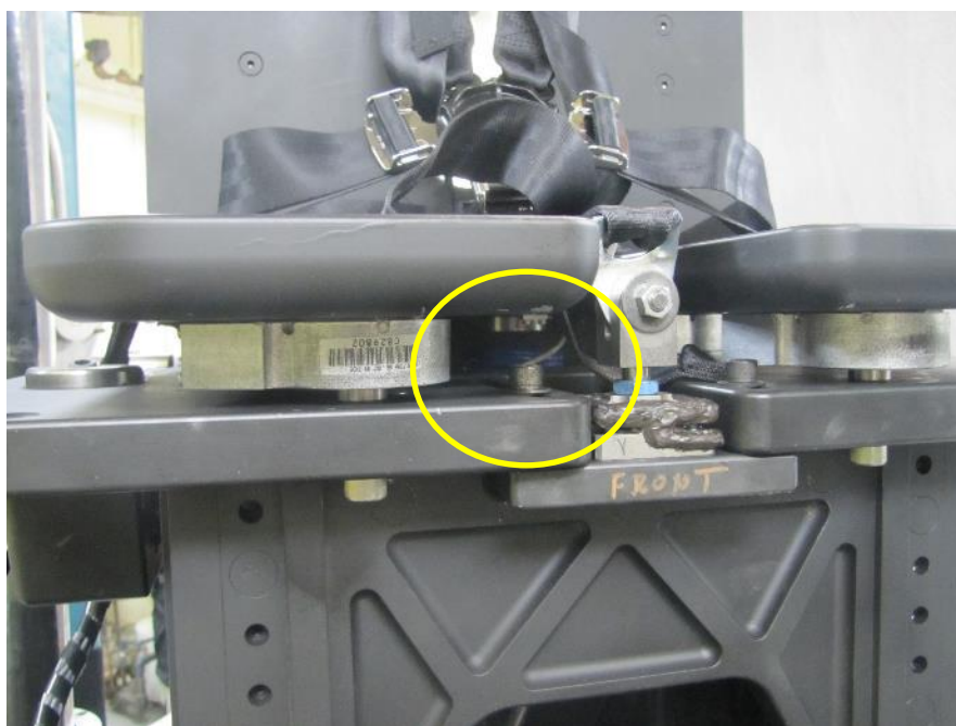
Figure 17. Location of Tri-axial Accel Array on WS2 Seat Pan
