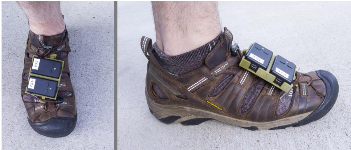
Figure 21. Right-Foot 2×1 Bracket Holding Two IMUs
