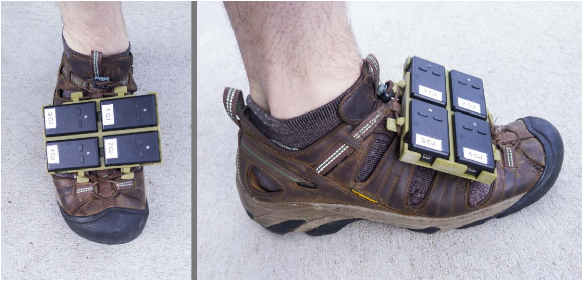
Figure 23. 2×2 Bracket Mounted with Four IMUs on Right Foot
