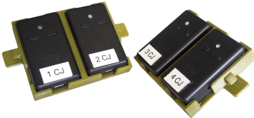
Figure 20. 2×1 Sensor Brackets, Left-Foot Bracket (Left) and Right-Foot Bracket (Right)
