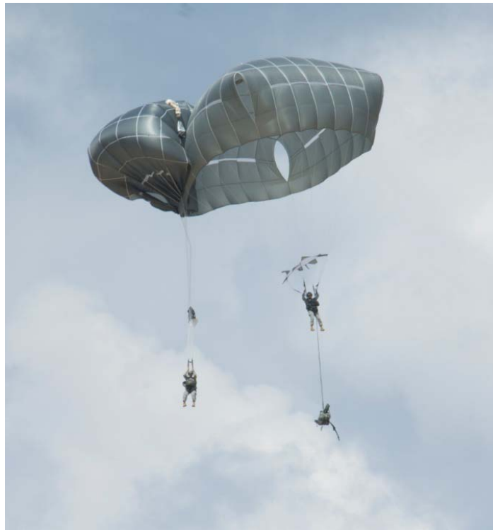
Figure 11. T-11 Corner Vent Entanglement. Source: Duncan (2016).
