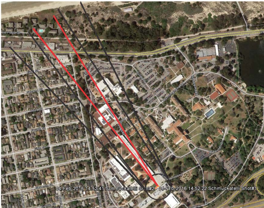
Figure 25. Electromagnetic Interference from a Cell Phone Causes the YEI TSS-DL to Return a 6.8-Degree Firing Azimuth Error
