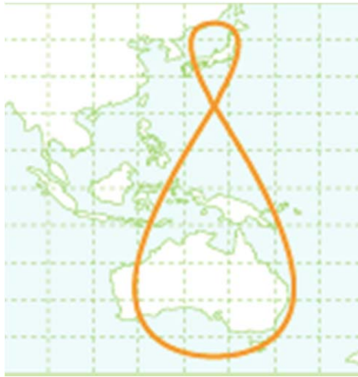
Figure 11. Asymmetric Figure-8 Geosynchronous Orbit Ground Track. Source: Japan Aerospace Exploration Agency (2003).
