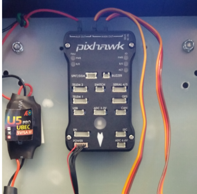
Figure 8. 3DR Pixhawk Autopilot Mounted in a Snowflake.
