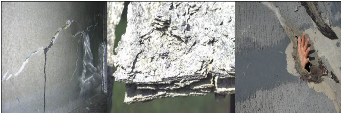
Figure 4. Stress Corrosion Cracking, Exfoliation, and Hole Formation, Respectively, due to Sensitization. Source: [4].
