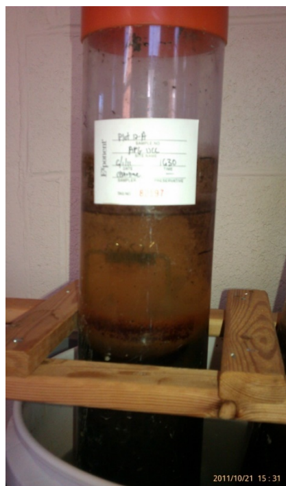
Figure 16. Laboratory set-up for intact cores from UCC. Strips of POM are used to assess the vertical gradient in resultant porewater concentrations.
