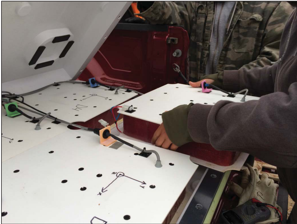
Figure 23. TEMTADS Coils Being Swapped
