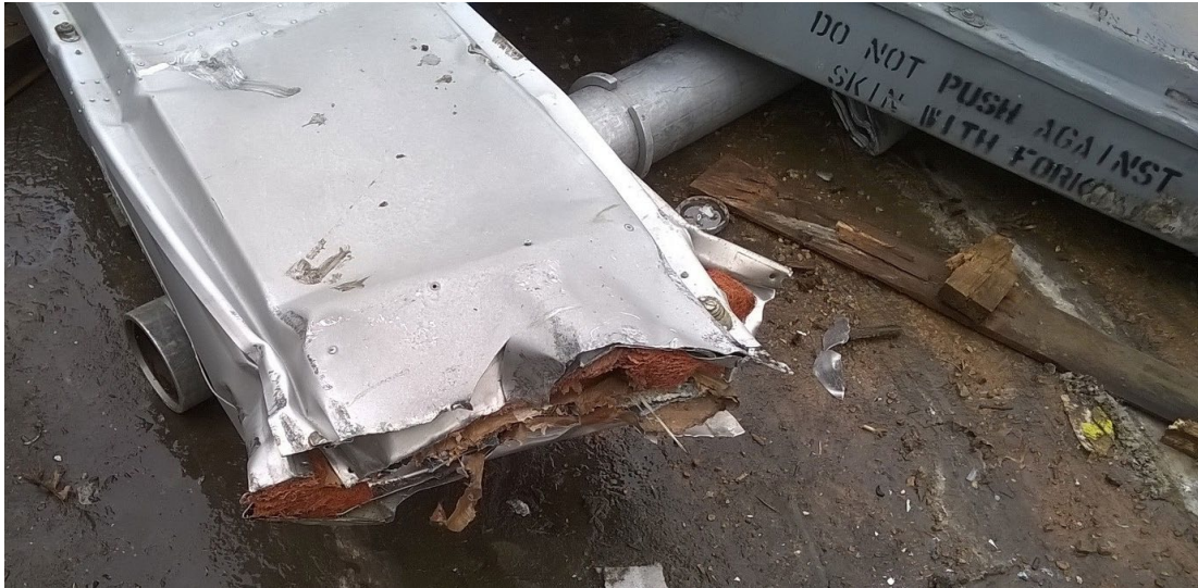
Figure 3. Mutilated Helicopter Blade and Holding Case Location: Holbrook, New York Source: DoD OIG
