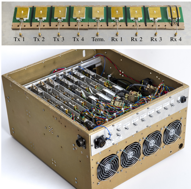
Fig. 2. ALSTAR prototype consists of a linear patch array with 4 transmitting and 4 receiving elements, and an 8-channel digital transceiver chassis.
