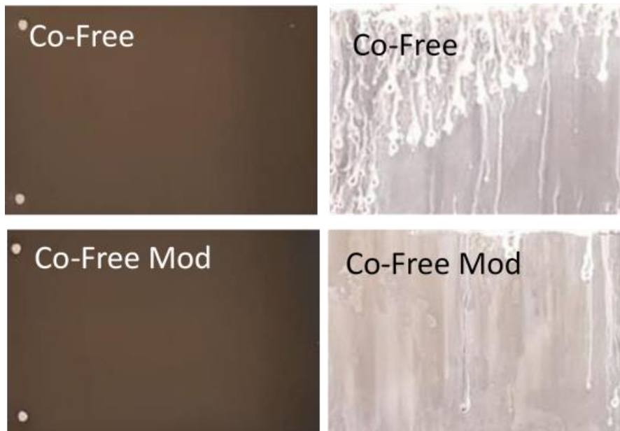
Figure 23. Optical images of Co-Free TCP and Co-Free Mod passivated ZnNi samples before (left) and after (right) 1000 hours of ASTM B117 neutral salt spray exposure
