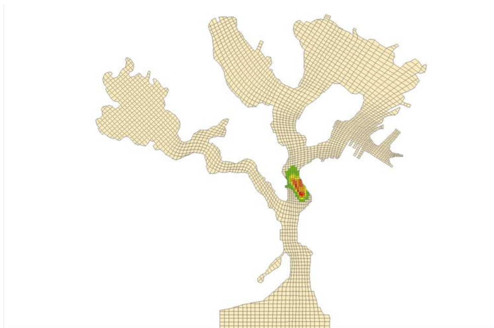
Figure 6-97. Initial dissolved copper concentrations at Oscar Pier surface layer for CH3D simulation at t = 0 after resuspension from prop wash (color key applies to Figure 6-97 through Figure 6-100).
