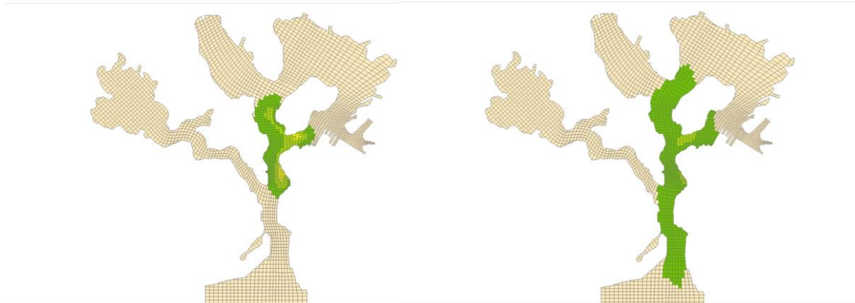
Figure 6-98. Figure 4-98. Simulated dissolved copper concentrations at Oscar Pier surface layer for CH3D simulation at t = 3 hours (left), and at t = 9 hours after prop-wash resuspension.
