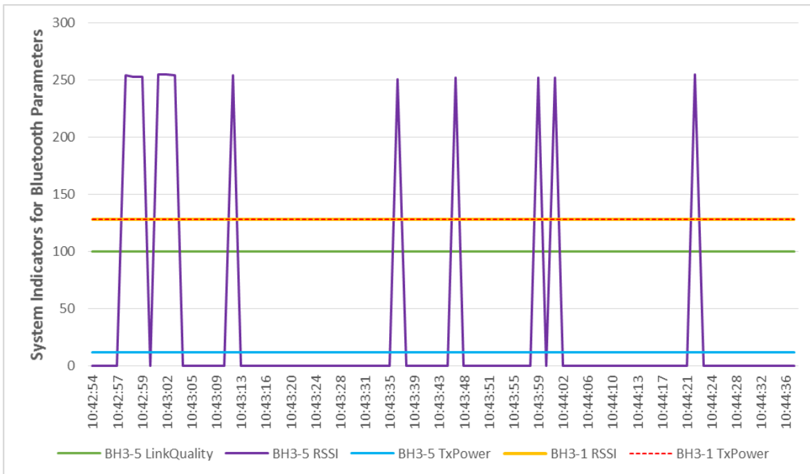
Figure 55. Phase 1: Omni data from MacBook: Bluetooth connection with BH3-1 and BH3-5 during two sensor bench testing
