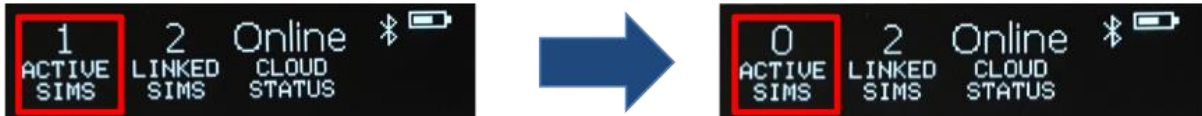
Figure 79. Phase 2b: SKYi display indicating that an active SIM-G sensor has lost connection
