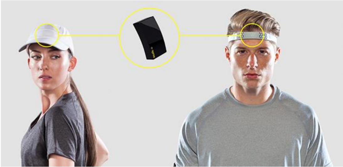
Figure 15. Example of a headband sensor that can measure heart rate and body temperature
