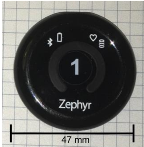
Figure 27. Zephyr BioHarness 3 sensor
