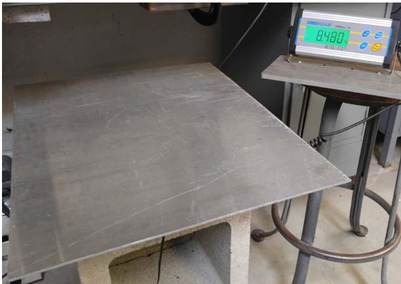
Figure 28. Electronic balance used to measure CFF thrust.
