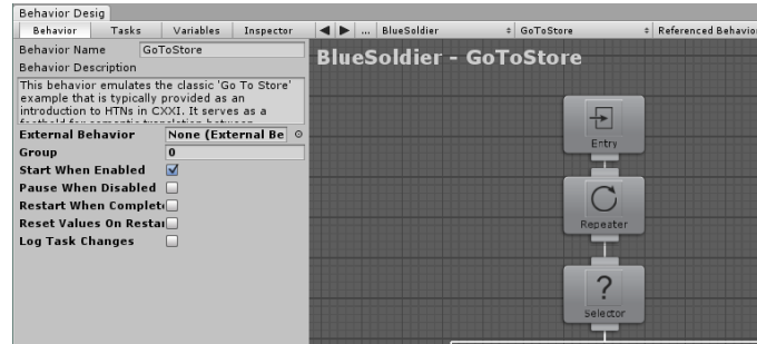
Figure 6.1: Placing a repeater node at the top of the tree or selecting the "Restart when complete" box will allow for emulation of a replan event.
