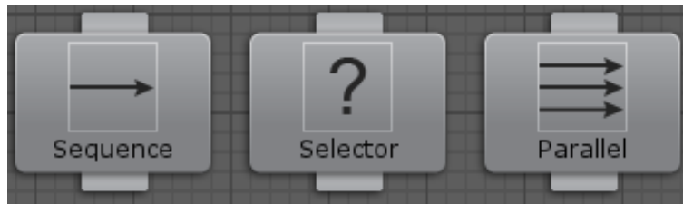
Figure 2.4: Three major types of composite nodes. Source: [24].
