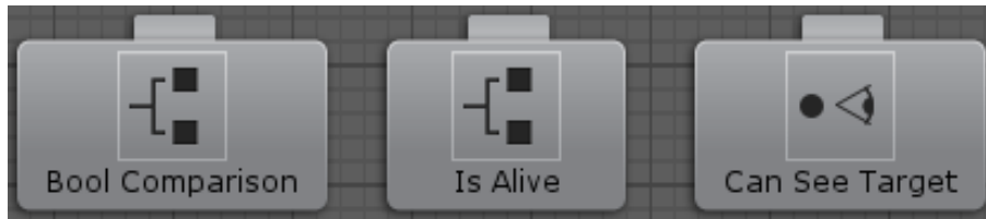
Figure 2.6: Examples of conditional nodes. Source: [24].
