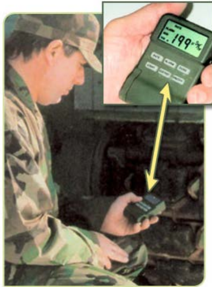
Figure 3. RGU-100 high sensitivity military pocket radiac
