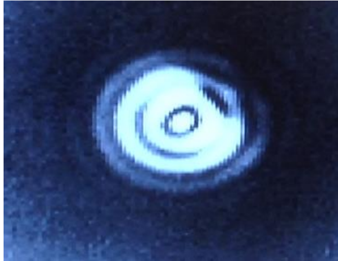
Figure 26. QCL Beam Captured by Microbolometer Camera.
