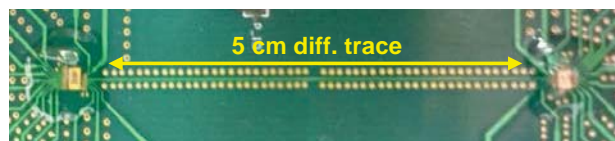
Figure 92: Top View of the Test Board with Separate TX/RX Connected with a 5-cm FR-4 Differential Trace
