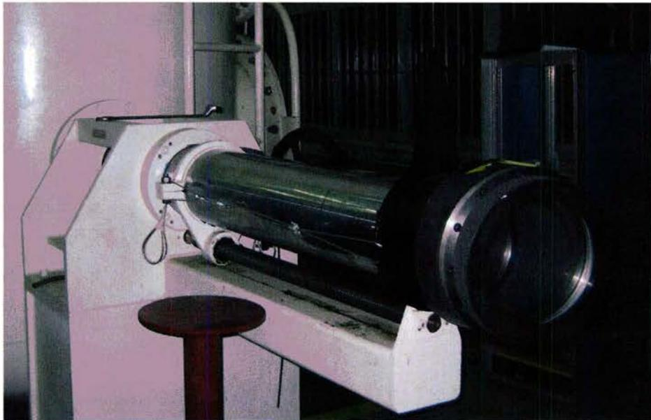
**Figure 3.2: Hollow HST sting with IR window and mount installed.**
