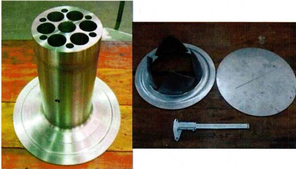
**Figure 3.3: ‘Petal catcher’ (left), and stainless steel diaphragms (right).**
