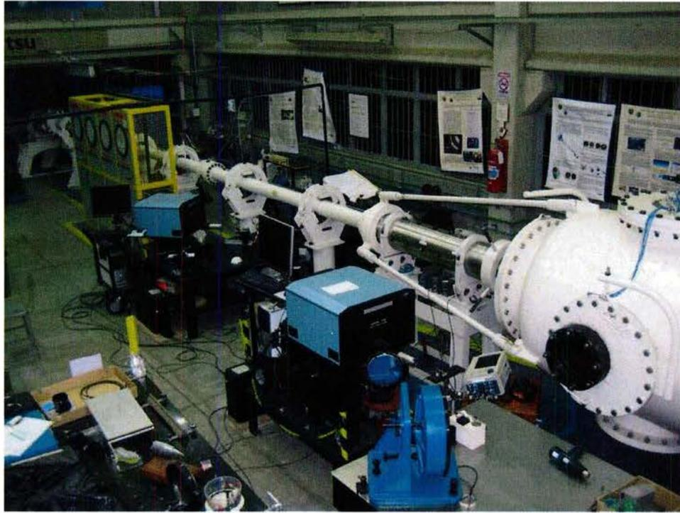
**Figure 3.1: T3 Hypersonic Shock Tunnel at the HTN-Laboratory of Aerothermodynamics and Hypersonics.**
