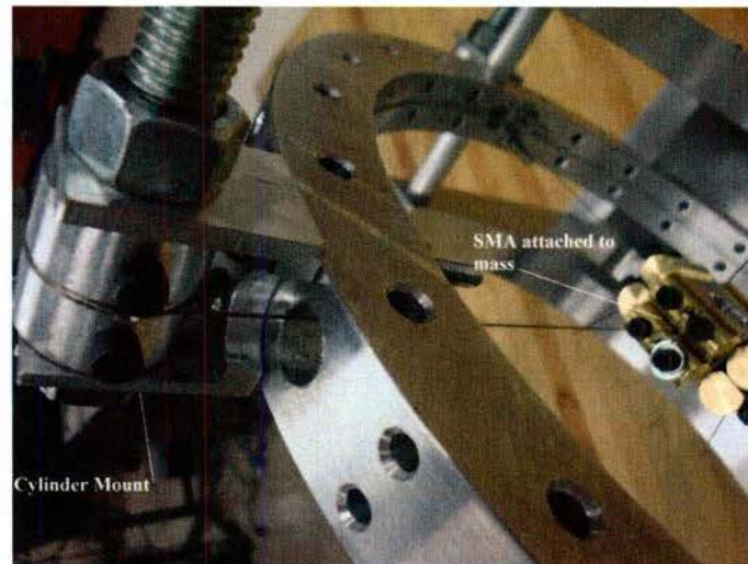
Figure 19 – Cylinder mounts for SMA wires
