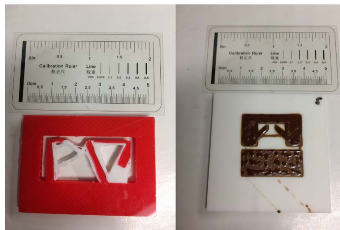
Figure 8. 3D printed parts of optimized designs
