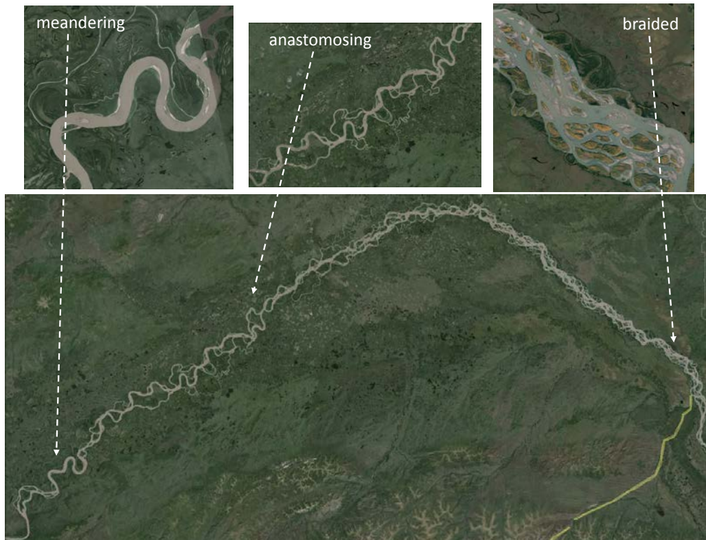
Figure 72. Examples of different channel planforms along the Yukon Flats portion of the Yukon River in central Alaska. (Images from Google Earth, Landsat, 4/2013 imagery date.)
