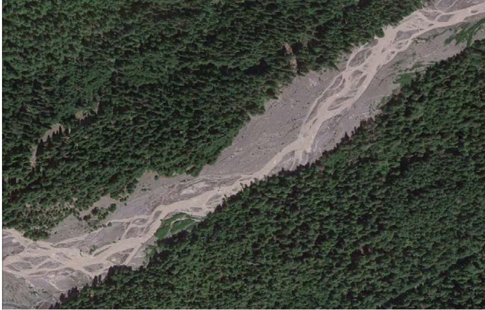
Figure 66. An example of a compound channel. Imagery of the White River, draining northeast from Mount Rainier in Washington (toward the upper right in both views). (A) In July, the channel is braided whereas (B) in September, the channel assumes a single-channel, more sinuous planform. (Map data from Google, DigitalGlobe.)
