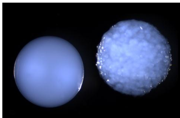
Figure 45. Alginate spheres of 2 mm diameter. The sphere on the left is comprised of \text{Ca}^{++} -crosslinked alginate only. On the right, a similar alginate sphere is filled with heparin-Sepharose microbeads with an average diameter of 90 microns.
