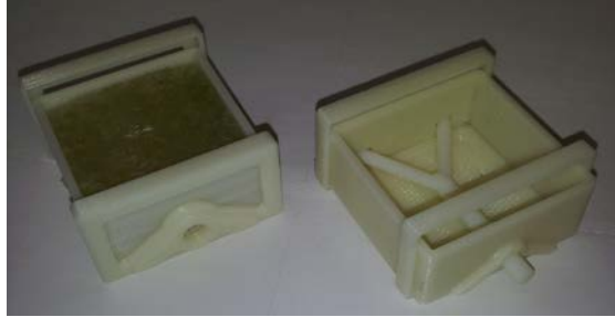
Figure. Mold designs and fabricated molds, with straight-vessel mold filled with gel.
