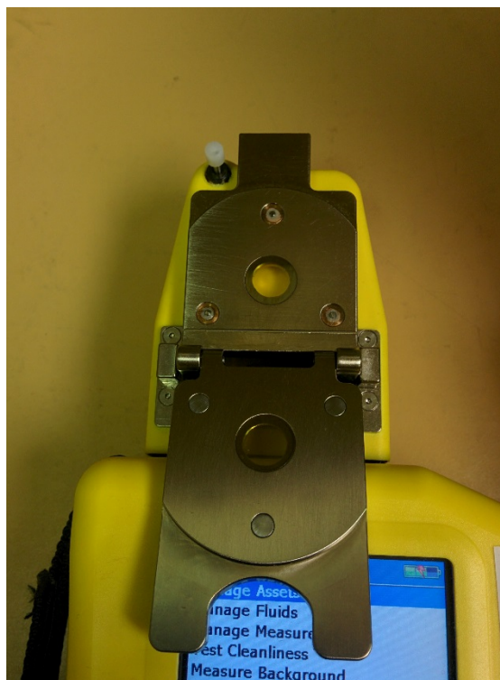
Figure 14. Quartz Windows of FluidScan Q1000 Used for Lubricant IR Analysis
