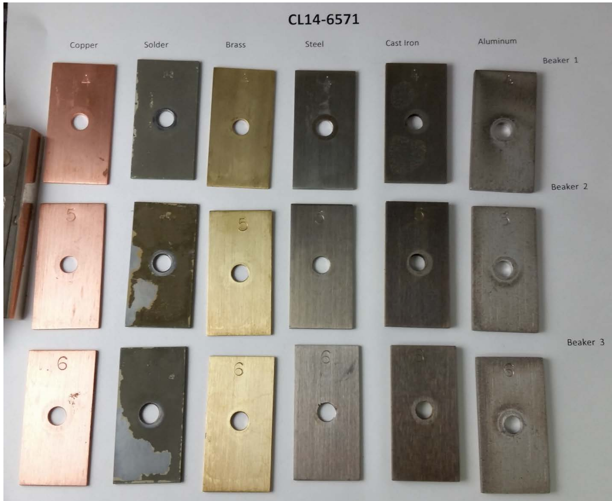
Figure 2. ASTM D1384 Coupons for Test CL14-6571 Extended Life Coolant #2
